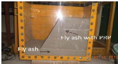
a) Fly ash with Plastic Recycled Polymer slope (Before failure)
