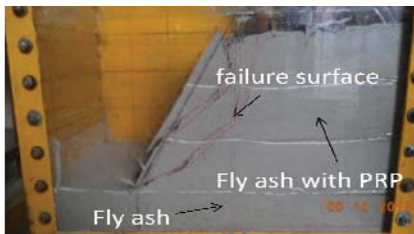
b) Fly ash with Plastic Recycled Polymer slope (After failure)
